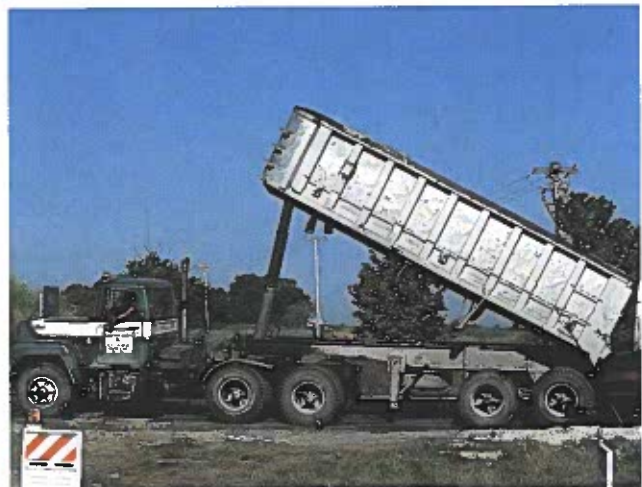
Figure 10-2. Hydraulic cylinders are able to lift heavy loads, such as the bed of this large dump truck.
