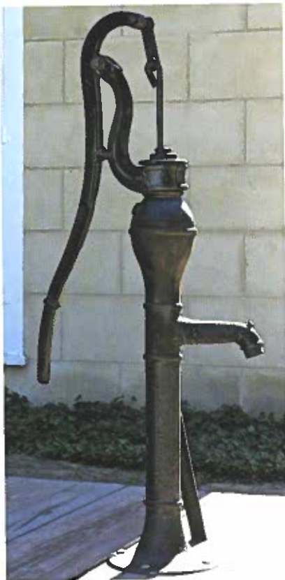
Figure 10-11. A simple hand-operated water pump. You may have used one like it.
