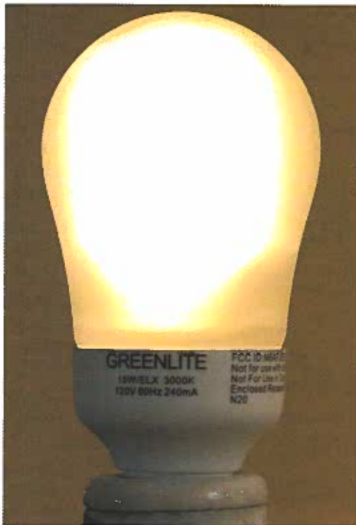
Figure 13-21. In a fluorescent lightbulb, ultra-violet (UV) radiation strikes a phosphor coating, generating visible light.
