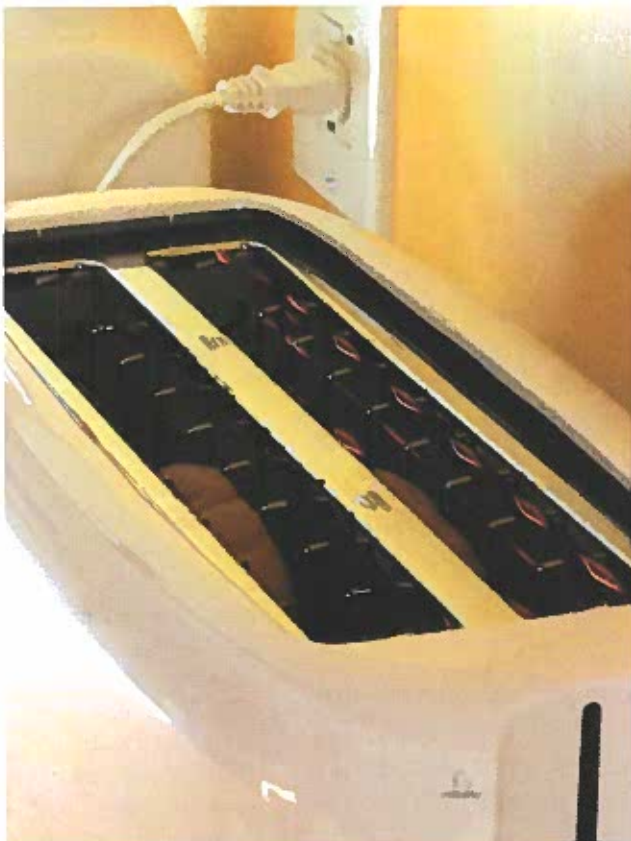
Figure 13-23. The heating element in this toaster is an example of energy inversion. Electricity flowing through the high-resistance heating element is converted to heat.
