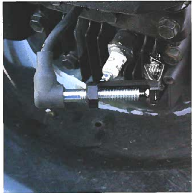
Figure 14-23. Using a spark tester to check for spark.
