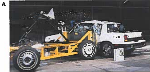
Figure 16-10. Structural testing. A—Automobile manufacturers conduct crash tests to determine the structural safety of their vehicles. (General Motors) B—Aircraft are crash tested to learn how fabrics and other materials resist burning. (National Aeronautics and Space Administration)
