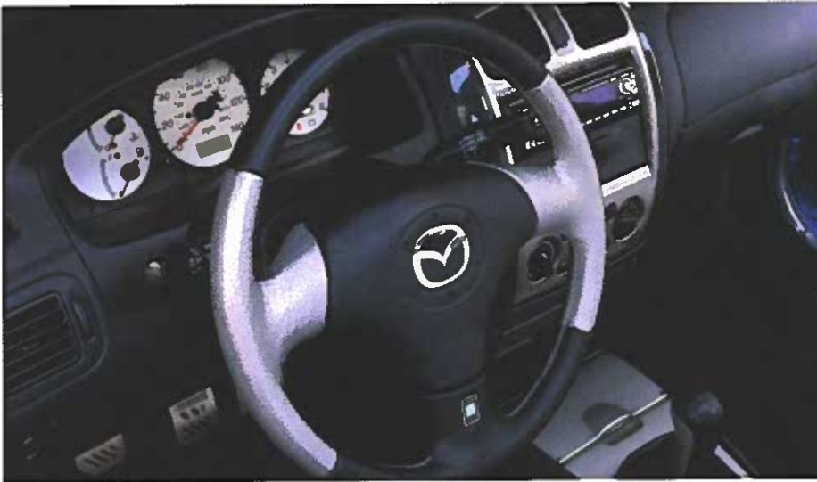
Figure 16-7. Directional control devices. A—A steering wheel for an automobile. (Mazda) B—An aircraft control stick. (Airbus) C—A “spinner” hand control for an industrial lift truck.
