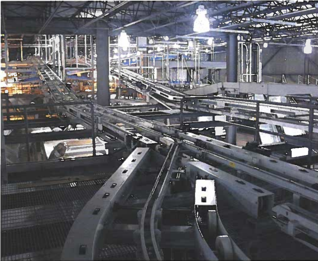
Figure 17-9. This complex conveyor system was built to move passenger baggage at DeGaulle International Airport in Paris, France. A conveyor system is a stationary pathway. (Siemens)
