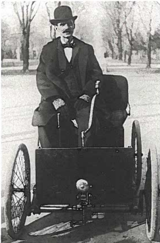
Figure 17-11. A two-cylinder, four-cycle engine powered Henry Ford's first car, which was invented in 1896. The car had an electric bell attached to the front to warn pedestrians.
