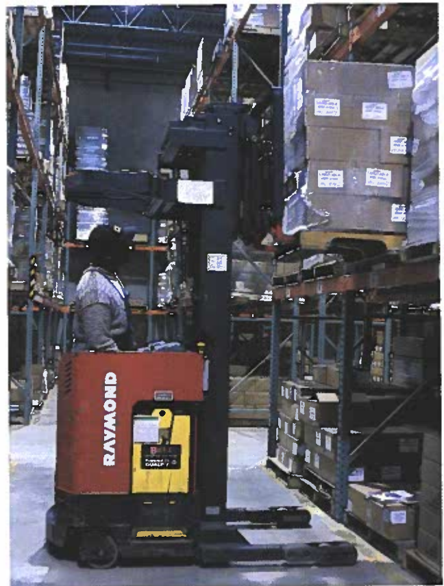
Figure 17-34. A forklift can move heavy pallet loads of goods from place to place and store them in stacks or in special shelving-type racks. Operator skill is important to prevent damage to the materials or storage racks.
