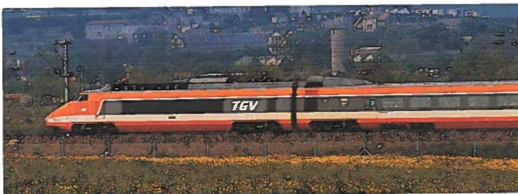
Figure 17-27. France's electric TGV ( train à grande vitesse , or high-speed train), operates at speeds well in excess of 200 miles per hour (mph). High-speed rail tracks must be built further apart than traditional tracks because of the turbulence when trains pass each other. They must also have fences on each side of the track to ensure that animals and debris do not enter the track area.
