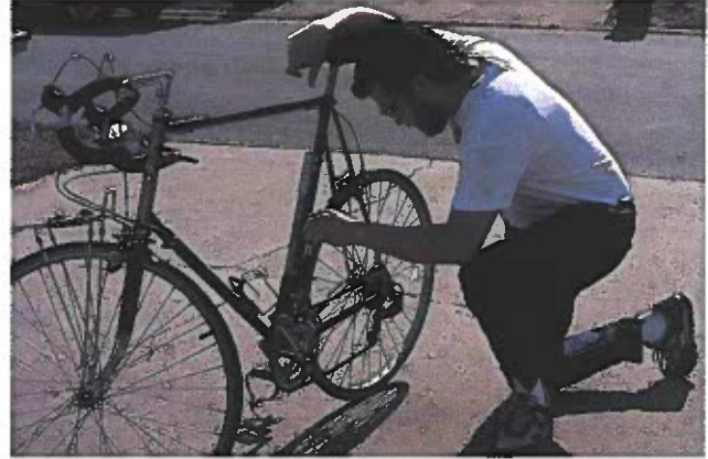
Figure 18-15. A bicycle has a drive system consisting of pedals attached to a large gear (sprocket). A chain transmits power from the sprocket to drive gears on the rear wheel. This is a simple form of drive system. (Howard Bud Smith)
