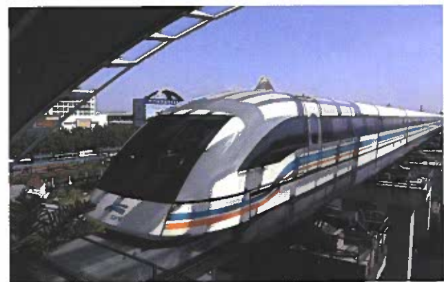
Figure 18-13. Linear magnetic motors on a magnetic levitation (maglev) train work with strong magnetic fields in the guideway to move the vehicle forward or backward. This train is pulling into a station in Shanghai, China. (Transrapid International, Inc., GmbH)
