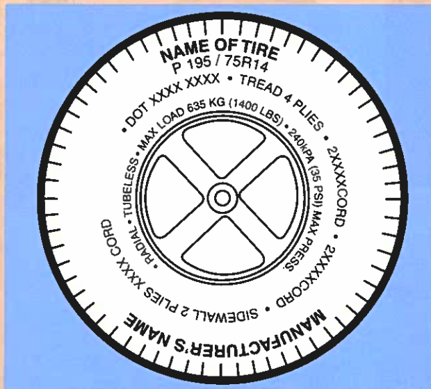
Figure 18-A. Tire information, such as its pressure rating, size, construction type, and maximum inflation, are molded into the sidewall.
