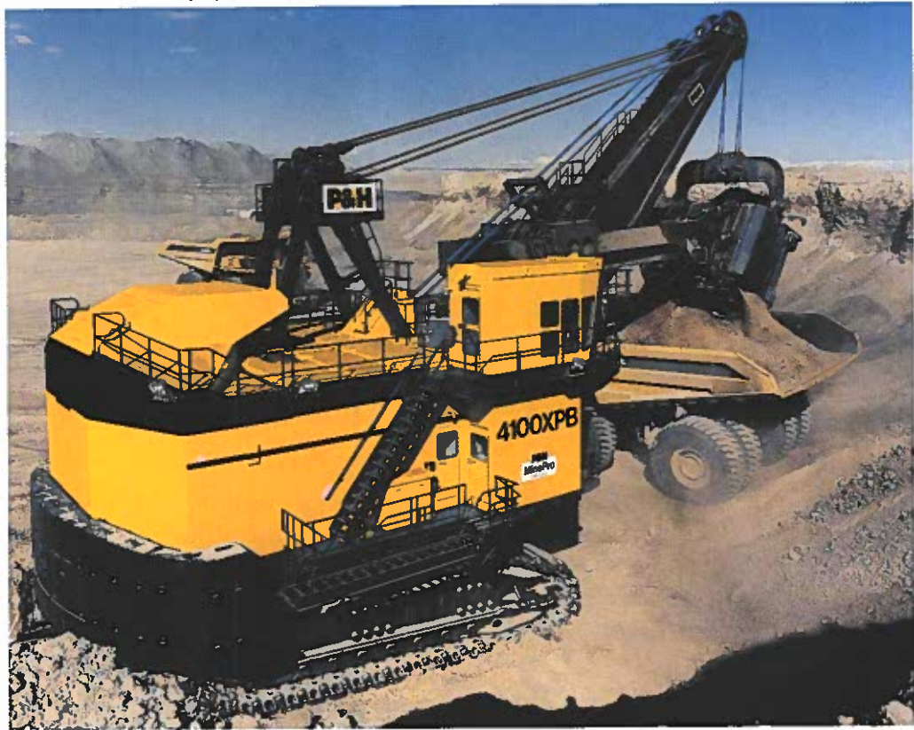
Figure 18-39. A tracked vehicle, such as this huge mining shovel, changes direction by altering the speed and direction of the two tracks. (P&H Construction Equipment)
