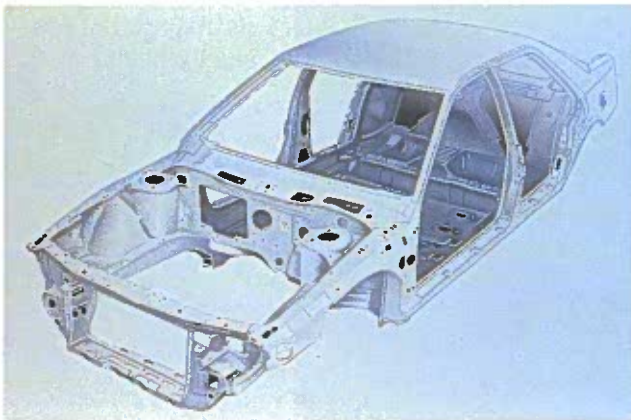
Figure 18-50. In unibody construction, the frame and body are combined in a single unit. (GM-Cadillac Motor Car Division)
