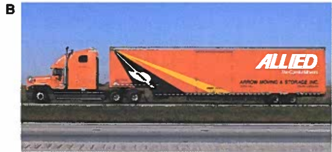
Figure 18-53. These trailers represent different types of cargo haulers found on the highways. A—A flatbed. (Fruehauf Trailer Operations) B—A closed (moving) van. C—A loose-cargo hauler. D—A tanker. (Fruehauf Trailer Operations)
