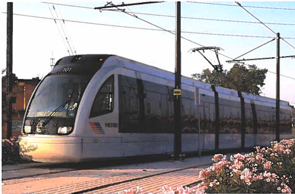
Figure 18-8. Overhead lines are the power source for electric trains used in many light-rail systems, such as this one in Houston, Texas. (Siemens)
