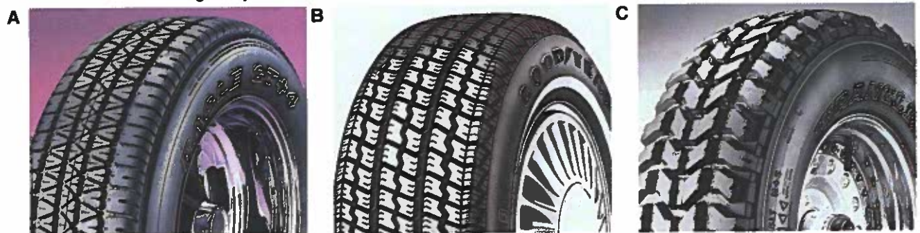
Figure 18-42. Tread designs vary depending on their purpose. A—An all-season performance tire. B—An all-weather highway tire. C—An off-road tire. (The Goodyear Tire & Rubber Company)
