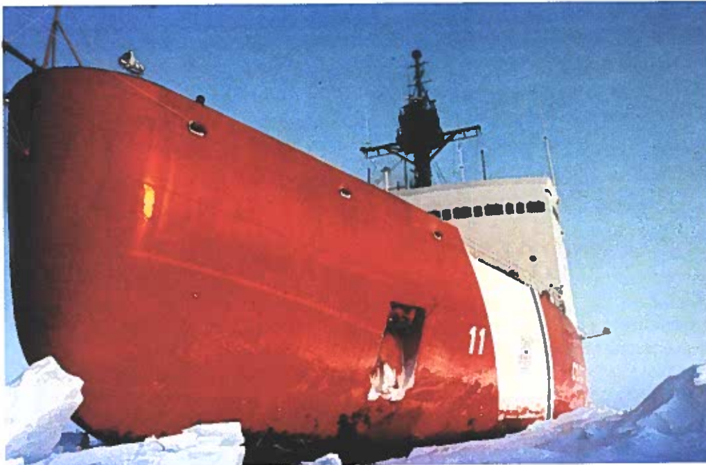
Figure 19-11. An icebreaker is a specialty vessel designed to perform a specific task. The U.S. Coast Guard cutter Polar Sea has a heavily reinforced bow to break through thick ice. (U.S. Coast Guard)
