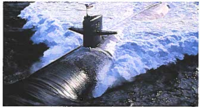
Figure 20-24. A submarine hull is designed and built to withstand tremendous pressure from the surrounding water when it submerges. (U.S. Navy)
