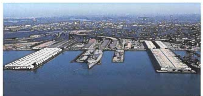
Figure 20-25. A modern deepwater harbor, which permits large vessels to tie up directly to a dock for loading or unloading. If a ship's draft is too great to tie up at the dock, it must anchor in deeper water. Smaller vessels called lighters are used to shuttle cargo between the dock and the anchored ship.
