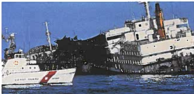
Figure 20-23. Watertight bulkheads are keeping this ship afloat, even though its bow was punctured in a collision, allowing water to flood some compartments. In such situations, the vessel is usually able to stay afloat and get to a port, where the hull can be repaired. All ships are fitted with collision bulkheads at the front. Areas where propulsion systems are located are also enclosed with bulkheads so this equipment is protected in the event of an accident. (U.S. Coast Guard)
