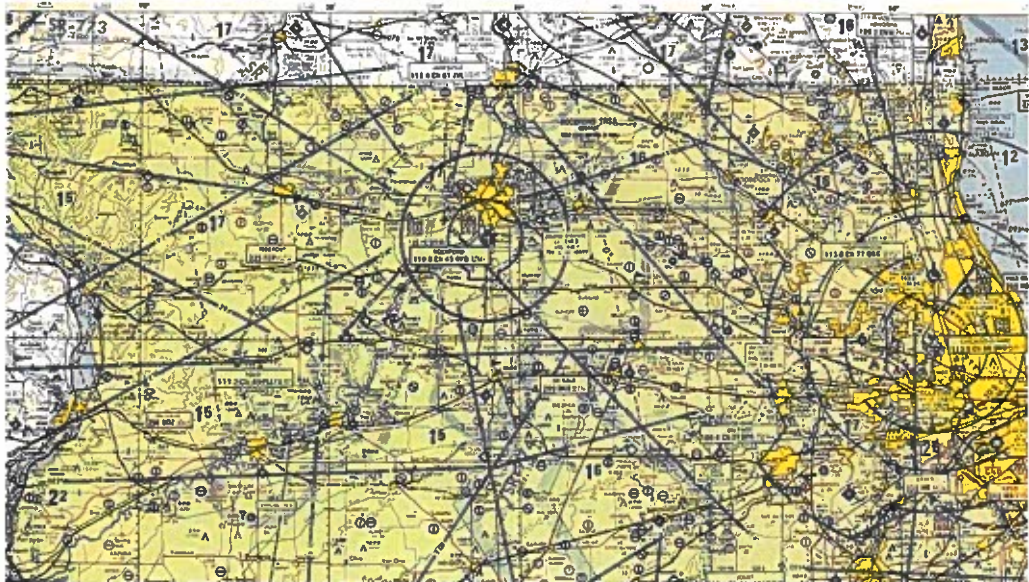
Figure 21-4. Airways are “highways in the sky” intersecting above very-high-frequency omnidirectional radio range (VOR) transmitters that provide location information. The circled area is the Rockford, Illinois VOR transmitter.
