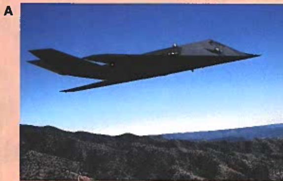
Figure 21-A. Stealth technology used for two different types of aircraft. A—An F-117 surveillance plane. B—The B-2 bomber. (U.S. Air Force)
