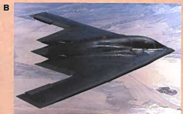
Figure 21-A. Stealth technology used for two different types of aircraft. A—An F-117 surveillance plane. B—The B-2 bomber. (U.S. Air Force)
