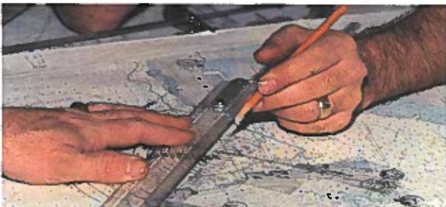
Figure 22-7. A navigation plotter is used with an aeronautical chart to plot the course of an aircraft. The plotter is made from clear plastic, and it combines a protractor with a straight edge marked with different scales.
