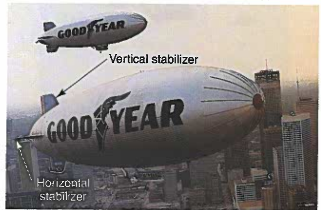
Figure 22-14. Horizontal and vertical stabilizers on a blimp function like rudders on a boat, turning the vehicle or making it rise or descend. (The Goodyear Tire & Rubber Company)
