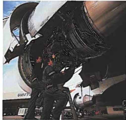
Figure 22-42. Inspections of aircraft engines and other systems and components are carried out on a regularly scheduled basis. These inspections are used to find faults that may cause engine, landing gear, electronic, or structural problems. The various inspections airplane support crews perform range from visual inspections to highly complex electronic inspections. (United Airlines)
