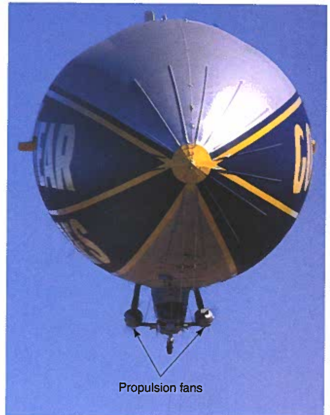
Figure 22-15. Propulsion fans mounted on the blimp's control cabin provide forward (or backward) motion and also can be swiveled to provide directional control. (The Goodyear Tire & Rubber Company)
