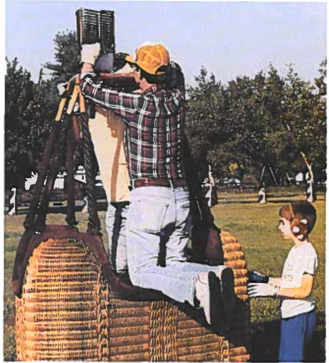
Figure 22-29. Because it is lightweight and shock resistant, wicker has traditionally been used for the baskets of hot air balloons.
