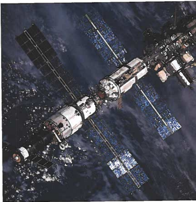
Figure 24-19. The International Space Station (ISS) is constructed from a series of interconnected modules produced by the United States, Russia, and Japan. Extending from one side of Unity are two Russian modules, Zarya and Zvezda . Each module has solar collectors attached to provide power to the station. Zarya serves as the control center, and Zvezda is the living quarters. Connected to the other side of Unity is the U.S. lab Destiny , which serves as a science lab. Other modules will be added to the ISS. (National Aeronautics and Space Administration)
