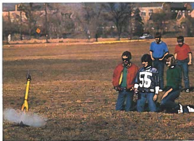
Figure 24-2. Model rockets use solid-fuel engines that are miniature versions of those that power full-size launch vehicles. This rocket is being launched during a high school technology education activity. (Estes)
