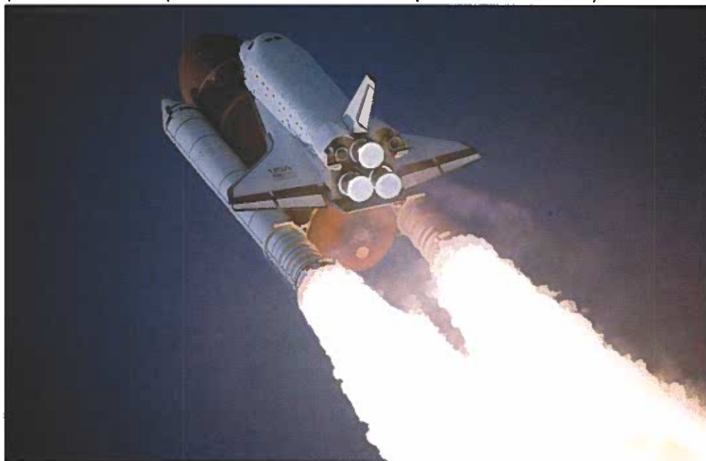
Figure 24-1. Tremendous power is needed to lift a space shuttle into orbit. In this view of a shuttle launch, the two solid rocket boosters (SRBs) and the three main engines on the shuttle itself are all operating, generating 7 million pounds of thrust. (National Aeronautics and Space Administration)
