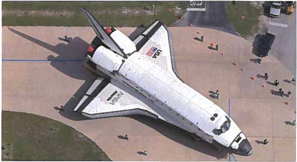
Figure 24-16. The space shuttle uses a triangular wing design known as the delta wing. This wing shape is most effective at supersonic speeds. (National Aeronautics and Space Administration)
