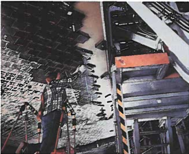
Figure 24-17. A technician installs high-temperature reusable surface insulation tiles on the wing of a space shuttle. Most of the tiles are 6 \times 6 in and range in thickness from 1" to 5". When heated, the tiles glow red, but they cool so quickly that within seconds, they are cool enough to touch. (National Aeronautics and Space Administration)
