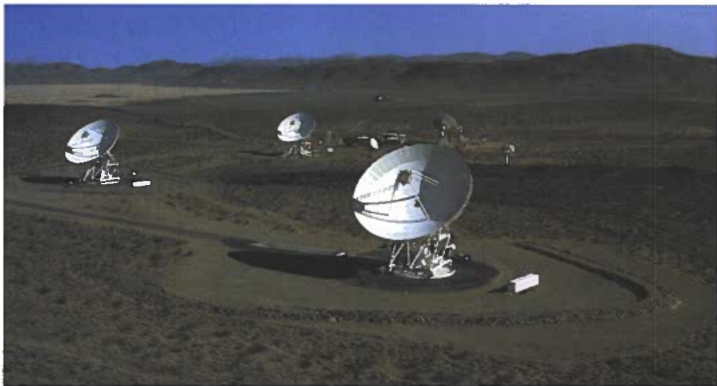
Figure 24-11. Deep Space Network (DSN) antennas at the Goldstone site in California's Mojave Desert are used for communication and to measure the Doppler shift when determining the velocity of a spacecraft. (National Aeronautics and Space Administration's Jet Propulsion Laboratory)
