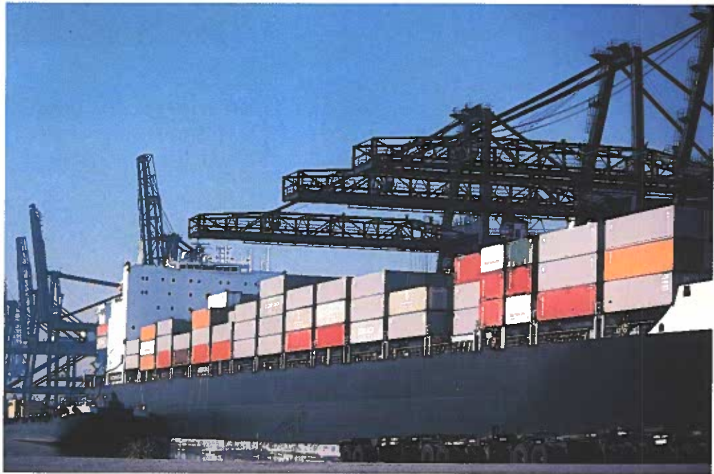
Figure 25-16. Giant cranes are used at intermodal ports to load containers on ships, unload them for storage, or transfer them to other means of transportation.
