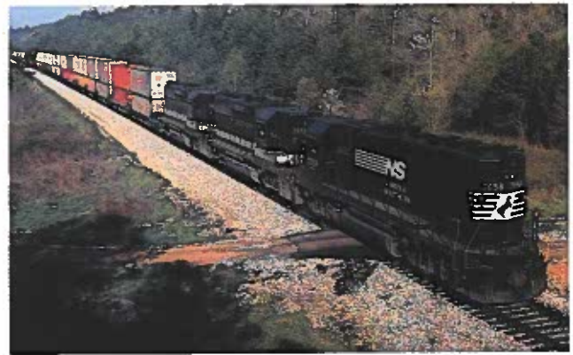
Figure 25-15. Rail transport. These containers have been stacked into well-type cars to be transported partway to their final destination. (Norfolk Southern Corporation)
