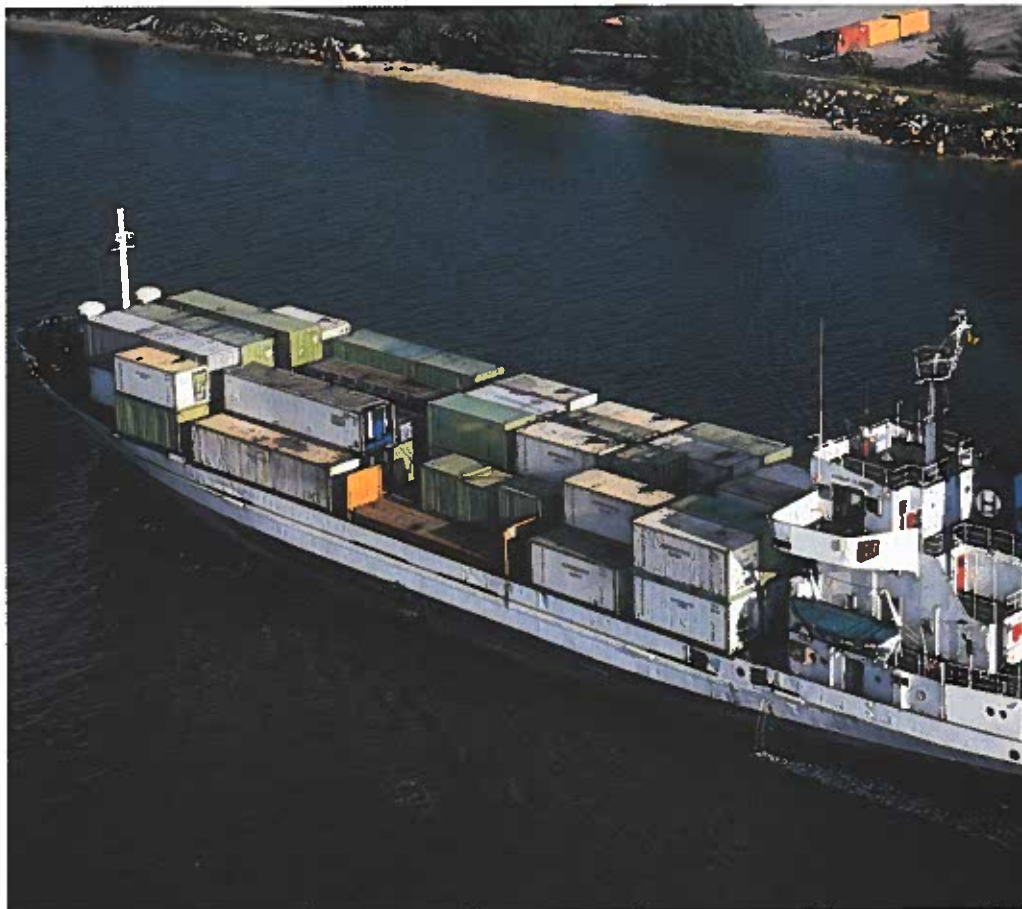
Figure 25-10. Containerships are designed to carry the maximum number of containers, both in their holds and stacked on deck.
