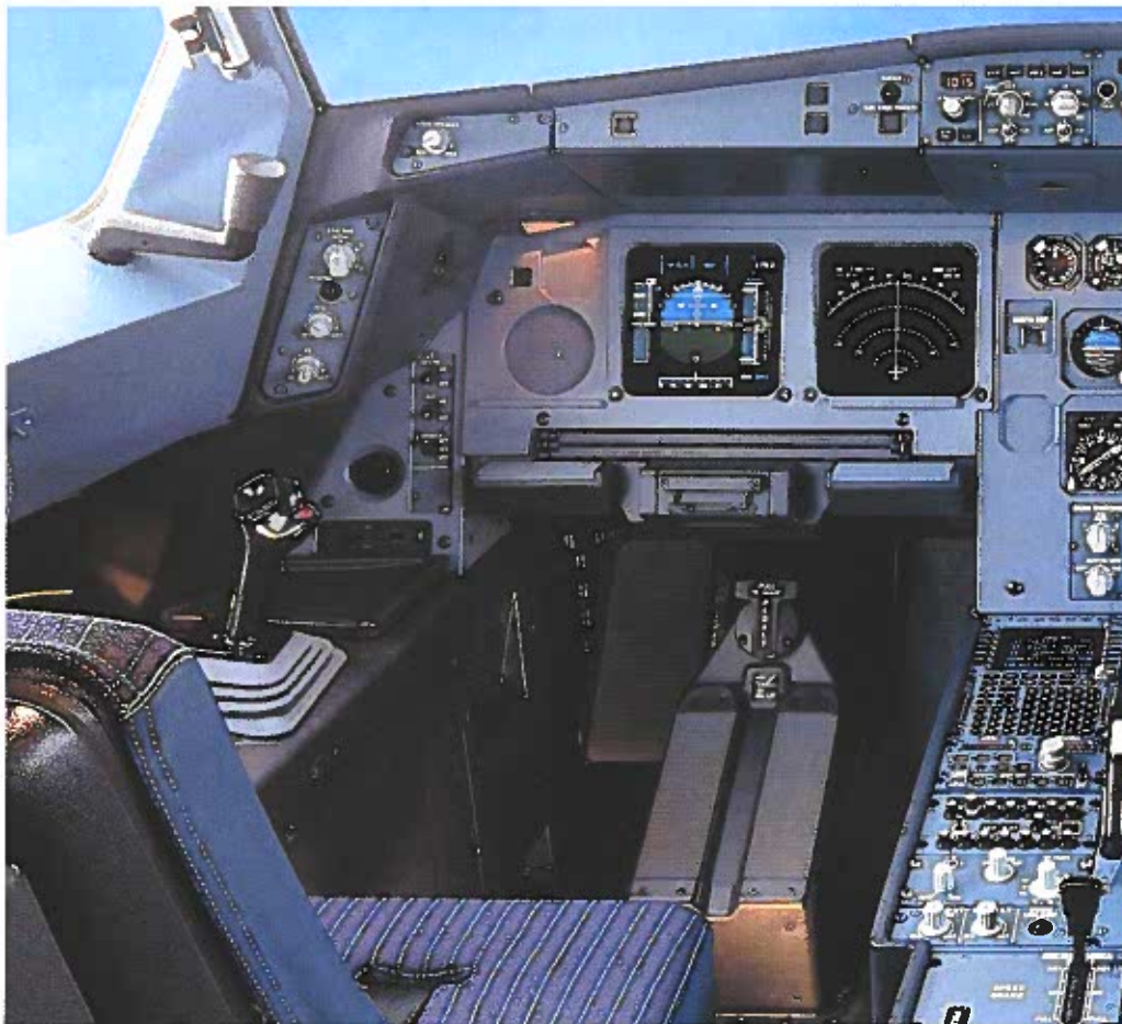
Figure 27-14. Digital displays have replaced many analog gauges and displays in the cockpits of both commercial airliners and smaller aircraft. This is the pilot-side instrument panel on a medium-range jet airliner. (Airbus)
