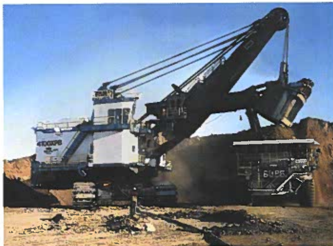
Figure 3-4. Coal located near the surface of the earth is mined by stripping away the dirt and rock above the coal seam. The exposed coal can then be broken up and shipped to electrical generating plants or other end users. Very large equipment, such as this shovel and truck, is used to mine with maximum efficiency. (P&H Mining Equipment)
