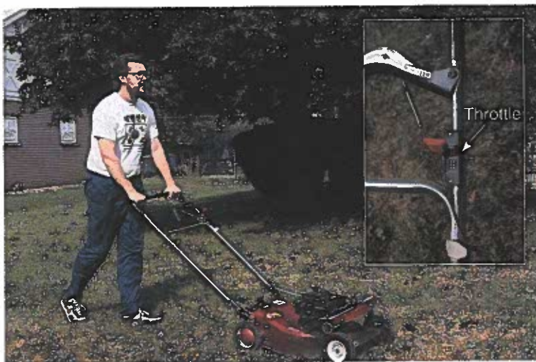
Figure 7-9. Control systems may be one-way or variable. The throttle of this lawn mower (inset) is used to vary the amount of power from the source (engine) to the load (cutting blade).
