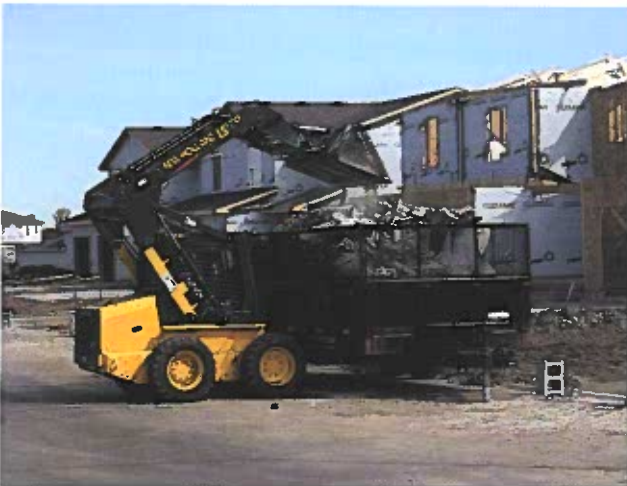
Figure 7-3. Many machines used in construction, such as this end loader, use hydraulics to transmit power and control machine functions.
