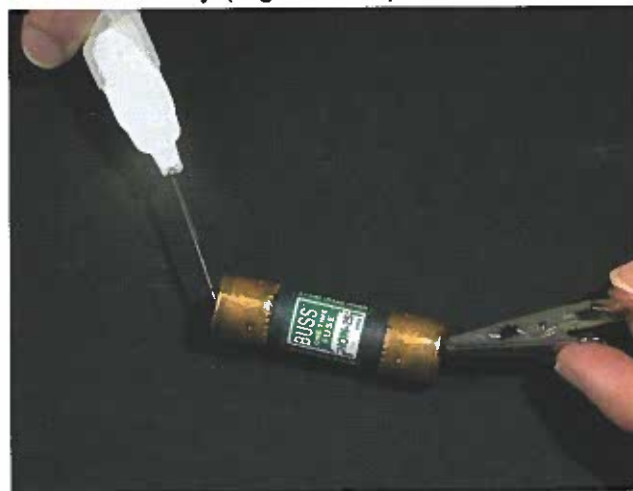
Figure 8-41. Using a continuity checker to see if a fuse is good or bad. A light or a beep indicates continuity (a good fuse).
