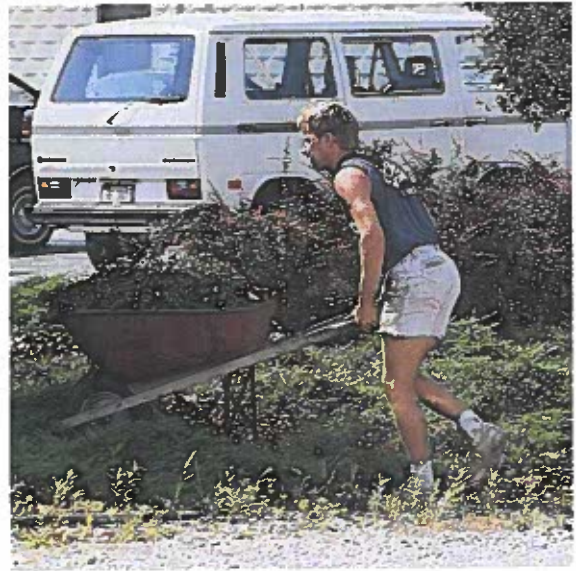
Figure 9-4. A wheelbarrow is a good example of a second-class lever. The fulcrum is the wheel, and the load is positioned between the wheel and the lifting force.
