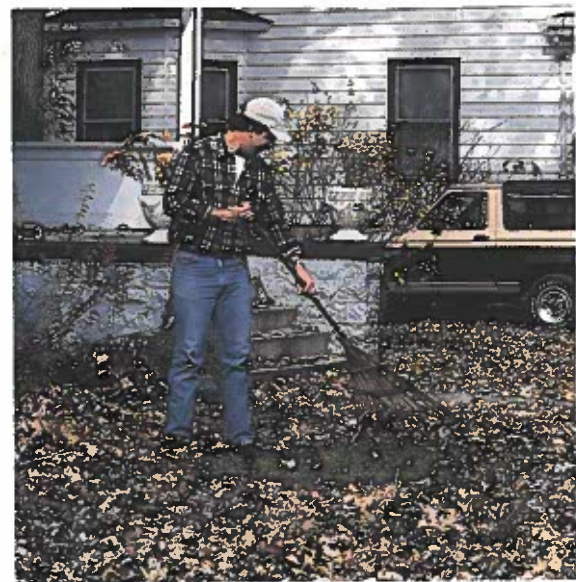
Figure 9-5. A third-class lever, such as this rake, is always a distance multiplier.
