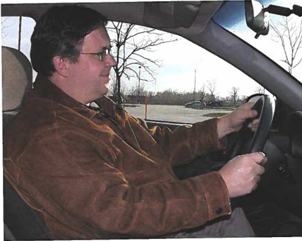
Figure 9-9. The steering wheel of an automobile is a type of lever. It multiplies the force used to turn the front wheels.
