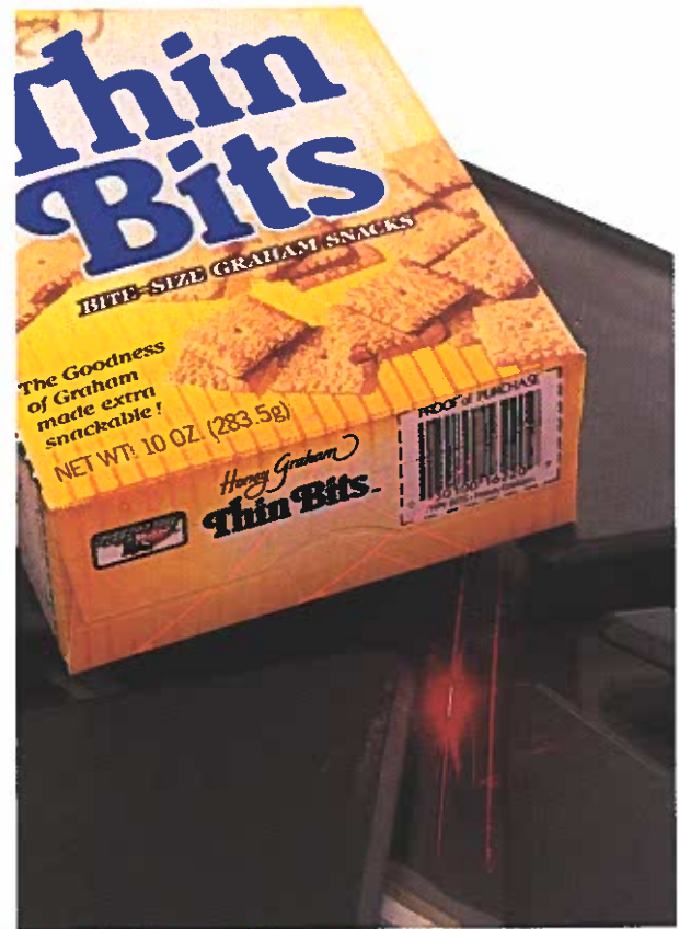
Fig. 1-2. Computer and laser technology make store checkout faster and easier. A laser beam scans the bar code on the package, then sends information to a computer about the product and its price.
