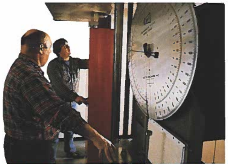
Fig. 6-3. Materials are selected for products based on information obtained by different types of testing. These people are testing the compression strength of cardboard corners.
