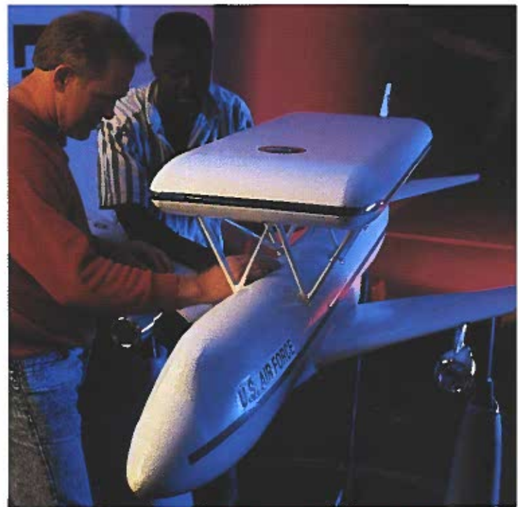
Fig. 6-2. Valuable information can be gathered by testing models or prototypes. Here, engineers are testing an aircraft design in a wind tunnel.
