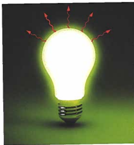
Figure 10-12. A light bulb is one example of energy conversion. Electrical energy converts into light energy and wasted heat energy.
