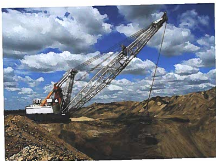
Figure 10-15. In open pit or surface mining, a dragline removes soil and rock to expose a coal deposit.
