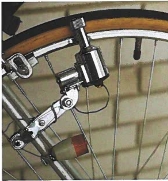
Figure 11-34. This bicycle light uses direct current supplied by the small generator. What advantage does this generator have over a light operated by a battery?
