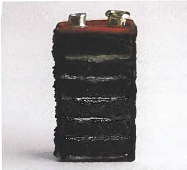
Figure 11-37. This cutaway of a 9 V battery shows that six 1.5 V cells are connected inside.
