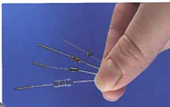
Figure 12-28. Resistors come in different shapes and sizes. They are often quite small.
