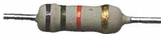
Figure 12-31. Use the chart in Figure 12-30 to calculate the value of this resistor.
