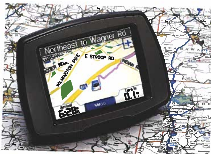
Figure 13-8. A GPS system is an example of a communication device that uses microchips to process information in real time.
