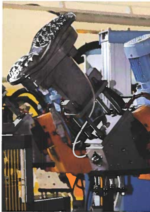
Figure 13-22. This industrial robot forms the soles of athletic shoes. The end effector, or working end, of the robotic arm is shaped to accept the shoe form.
