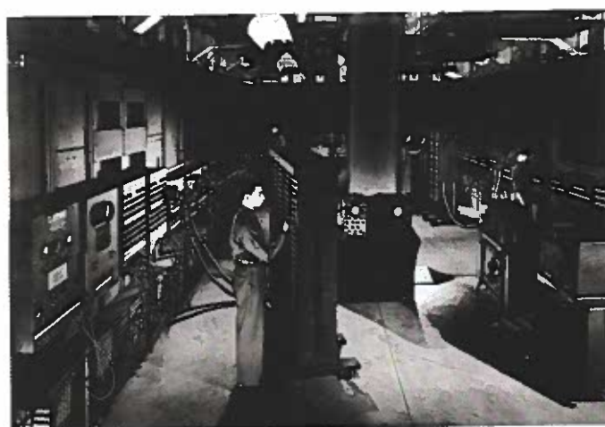
Figure 13-16. ENIAC stands for “Electronic Numerical Integrator and Computer.” It was designed to calculate ballistic firing tables. However, it was fully programmable, so it could perform many other tasks as well.
