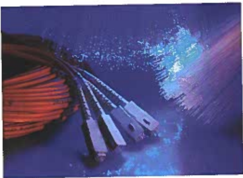
Figure 13-9. Fiber optic cables carry information coded as pulses of light. They can transmit data faster than copper wire, and they have a higher capacity.
