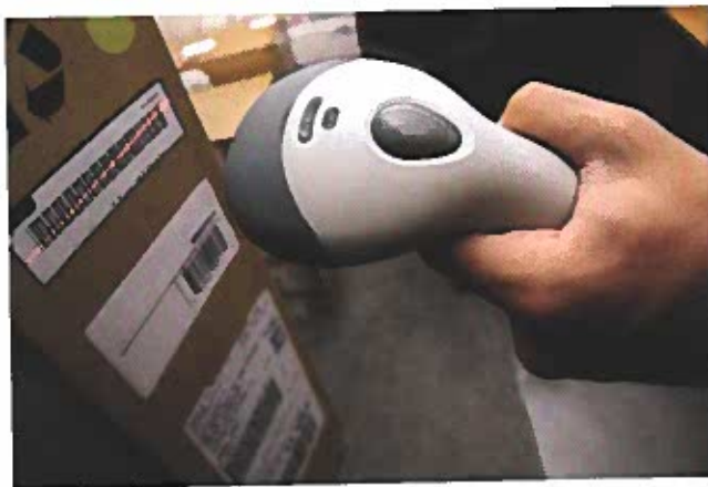
Figure 13-18. A bar code contains encoded information about a specific product. Warehouse workers often use bar code systems to help track orders and inventory.
