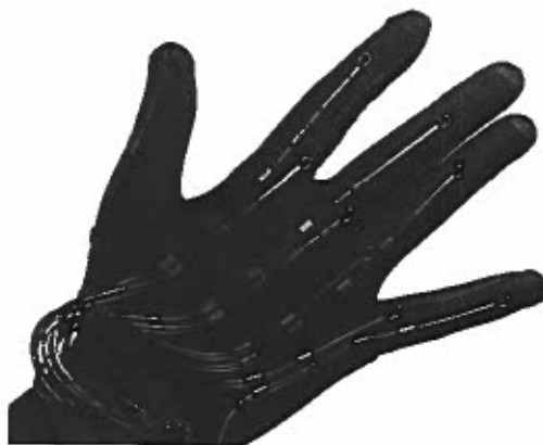
Figure 13-25. The sensors on a haptic glove allow you to touch objects in a virtual world.
