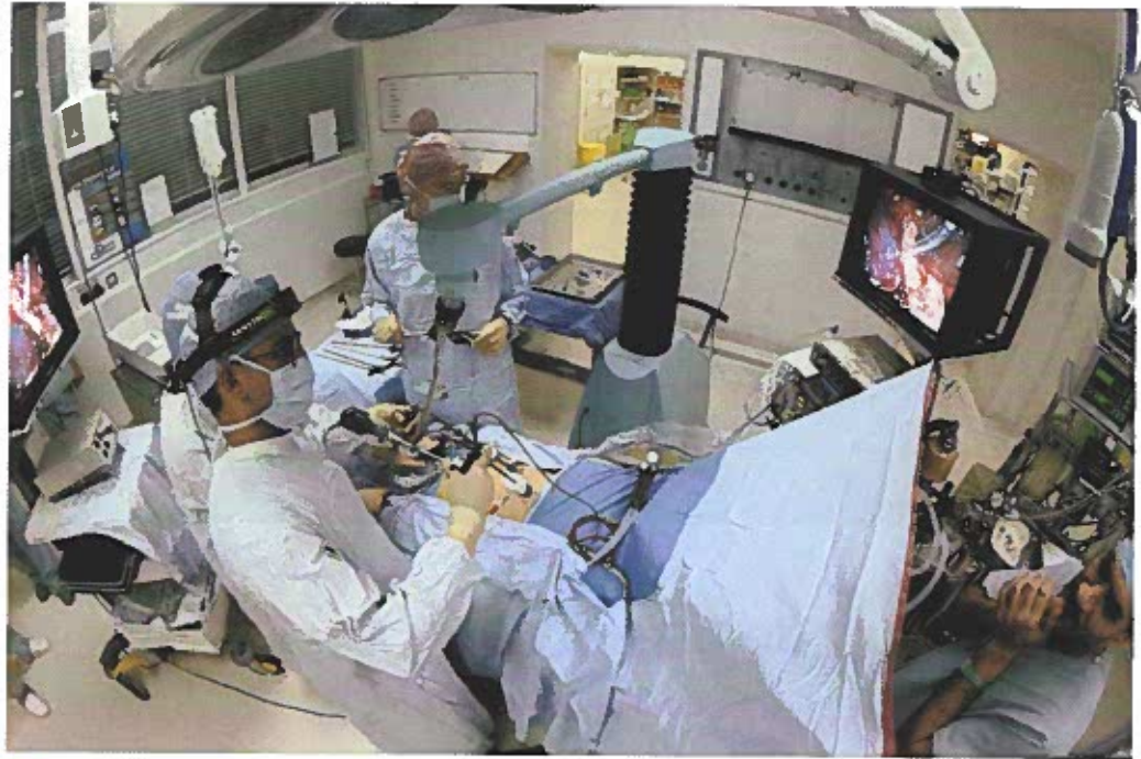
Figure 14-8. This surgeon is using a foot switch and special headband to control a robot, which holds and directs the tiny camera inside the patient's body.
