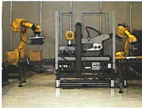
Figure 15-11. These robots automate the final packing and shipping of manufactured items.
