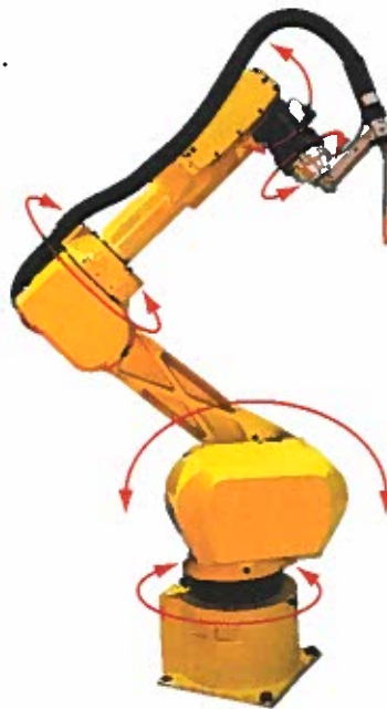
Figure 15-9. This industrial robot has five degrees of freedom.
