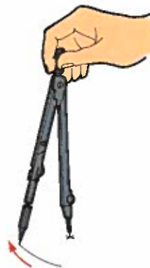
Figure 3-30. When using a compass, draw circles or arcs lightly at first. Make repeated turns to darken the line.
