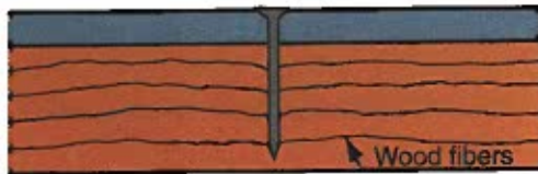
Figure 5-15. When a nail is forced into wood, the compression of the wood fibers and friction between the wood fibers and the nail hold the nail in place.
