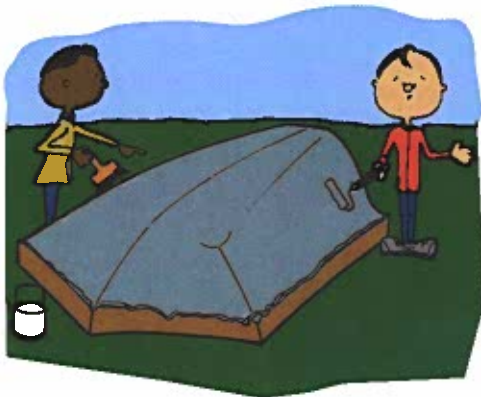
Figure 5-13. Molding fiberglass on a form, such as this boat, is called a lay-up .
