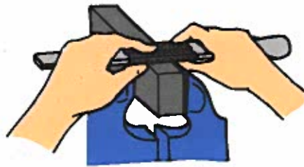
Figure 5-44. One way to use emery cloth on metals is to wrap the cloth around a file.
