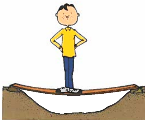
Figure 6-10. A person standing on a plank causes the plank to bend. Bending causes compression on the top surface of the plank and tension on its bottom surface.
