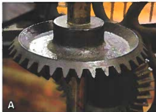
Figure 8-48. A—Bevel gears change the direction of the applied force. B—A hand drill uses bevel gears.
