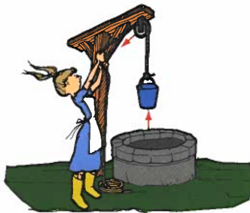
Figure 8-1. Changing the direction of applied force makes it easier to lift heavy objects. As the woman pulls down on the rope, the pail moves upward.
