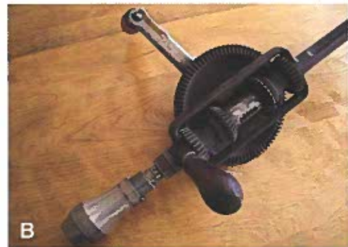
Figure 8-48. A—Bevel gears change the direction of the applied force. B—A hand drill uses bevel gears.
