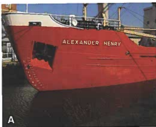
Figure 8-30. We use the wedge in many products. A—The wedge-shaped prow (front) of a ship cuts easily through the water. B—The teeth on the bucket of a backhoe are wedge-shaped to enter the soil more easily.
