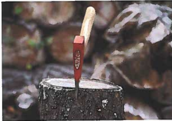
Figure 8-29. Because of its shape, an axe enters material easily and can split it apart.
