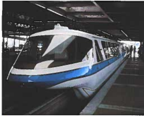
Figure 8-62. One of the effects of streamlining is to reduce air drag, which is a form of friction.
