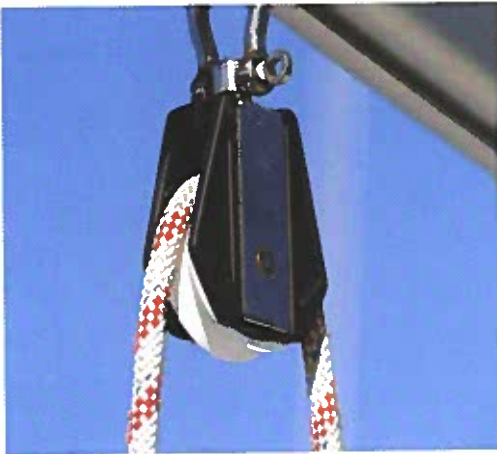
Figure 8-17. A simple pulley changes direction once.
