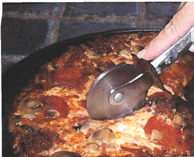
Figure 8-25. A pizza cutter is a form of wheel and axle. Where are the effort, fulcrum, and resistance located?
