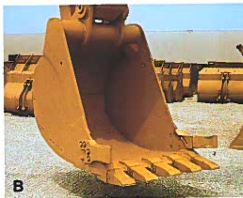
Figure 8-30. We use the wedge in many products. A—The wedge-shaped prow (front) of a ship cuts easily through the water. B—The teeth on the bucket of a backhoe are wedge-shaped to enter the soil more easily.
