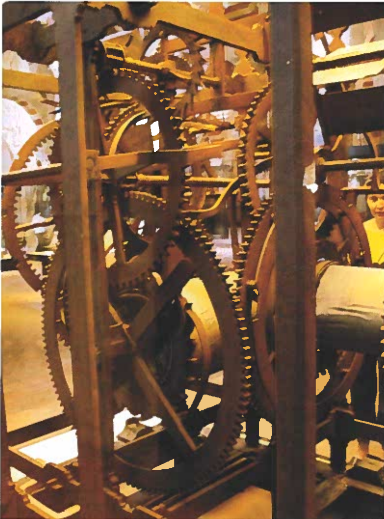
Figure 8-36. Gears are similar to pulleys, except they have teeth that prevent them from slipping.
