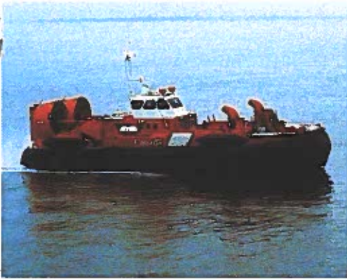
Figure 8-61. Hovercraft use a cushion of air to reduce friction.
