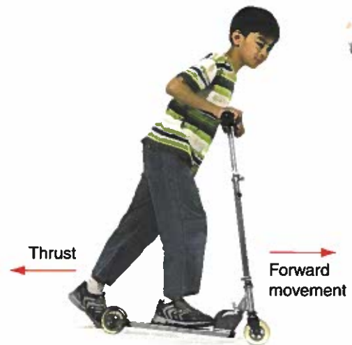
Figure 9-27. Pushing backward against the ground with one foot creates thrust. This pushes the scooter and the boy forward.
