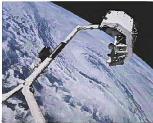
Figure 9-40. The Space Station Remote Manipulation System (SSRMS) contributed to the International Space Station by the Canadian Space Agency.
