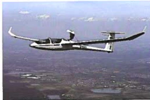
Figure 9-12. This glider has a retractable engine that allows the aircraft to be self-launching. The engine also provides a back-up source of power for those times when it flies too low.
