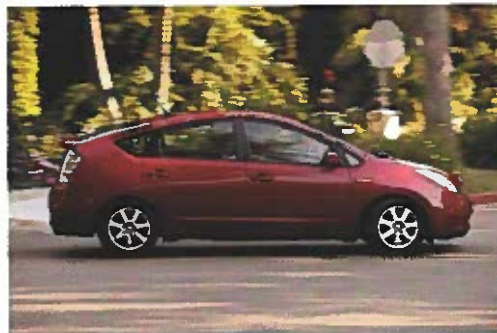
Figure 9-32. Gas-electric hybrid cars such as this Toyota Prius employ a regenerative braking process, which can provide power to the battery or directly to the electric motors.
