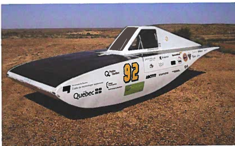
Figure 9-35. Eclipse VI was a competitor in the 2009 North American Solar Challenge. The solar cells, which cover most of the upper body surface, convert the energy in light into electrical energy.
