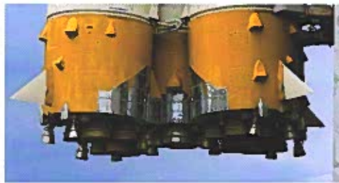
Figure 9-31. Because space has no oxygen, rockets that travel in space must carry both fuel and oxygen for combustion.
