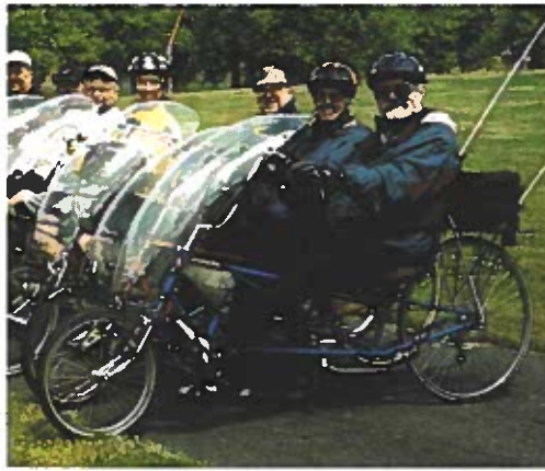
Figure 9-18. Wind resistance is a major force that must be overcome by a cyclist. What three things have been done to these bicycles to lower wind resistance?
