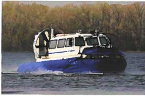
Figure 9-7. Hovercraft fly just above the water's surface on a cushion of air.
