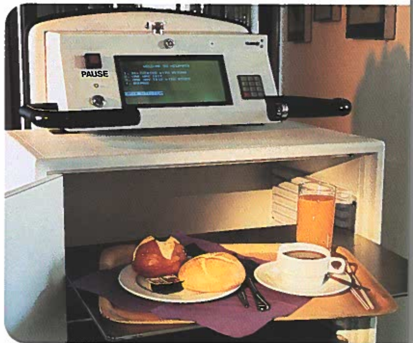
Fig. 10-6. This robot used to deliver food and other items in a hospital navigates by means of a map stored in its memory. In what ways would a robotic delivery system make your own life easier?
