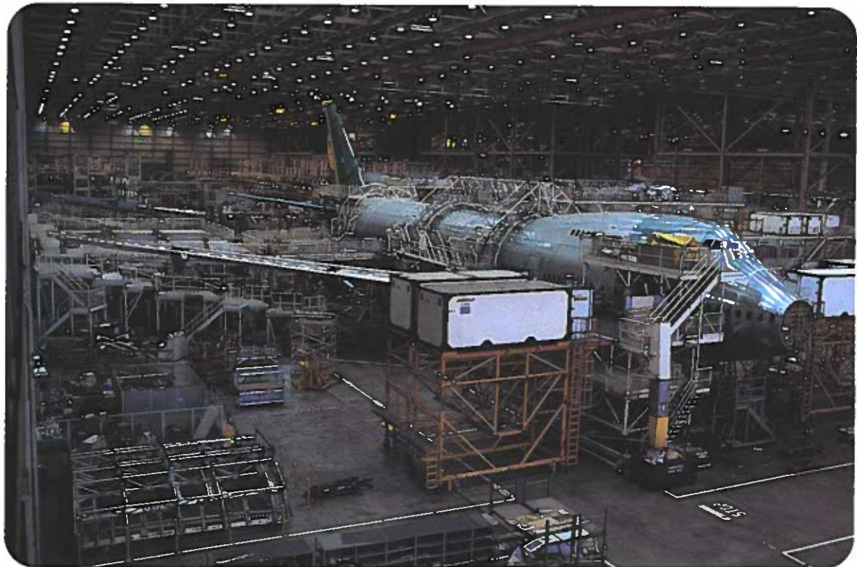
Fig. 10-3. Large airplanes like this Boeing 747 are made with custom production methods. What other types of products are still produced this way?
