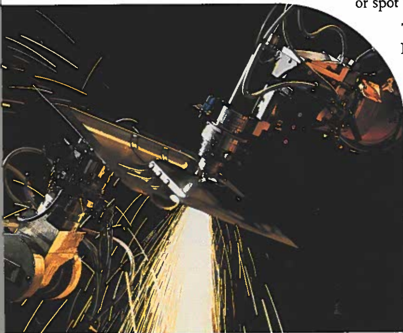
Fig. 10-7. Metal produces a shower of sparks as a robot cuts through it using a laser. Why do you think a robot would be ideal for this kind of job?
