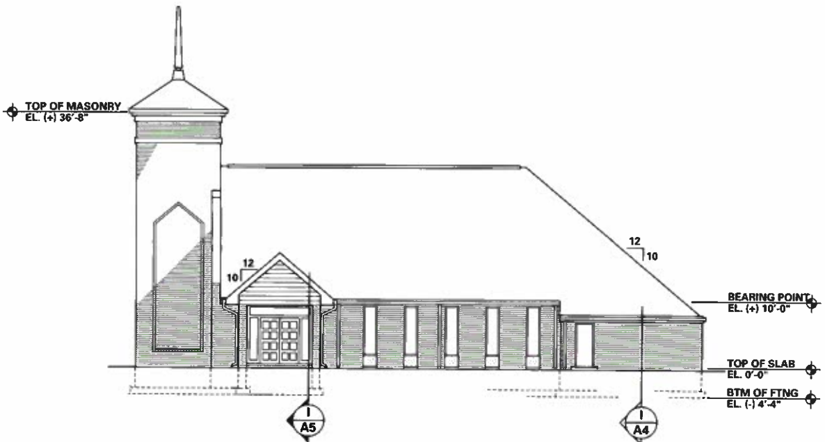
Fig. 12-6. This elevation shows the front of a church. What is the height of the tower masonry?
