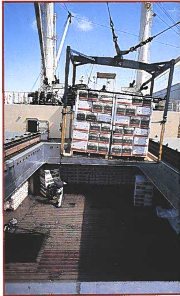
Fig. 14-11. A crane lowers cargo into the hold of a ship. Some method is usually used to hold the cargo in place. What do you think could happen if the cargo in a ship were to suddenly shift?
