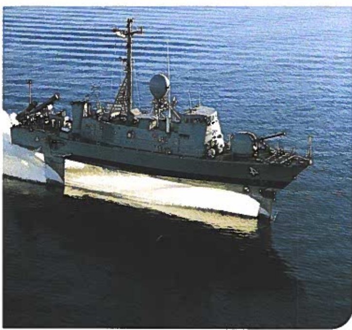
Fig. 14-9. Hydrofoils skim over the water thanks to the lift created by the hydrofoil “leg.” The shape of a hydrofoil is similar to that of an airplane wing.
