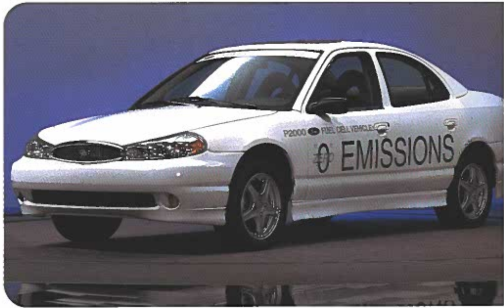
Fig. 14-2. This Ford P2000 automobile uses both diesel and electric power. It is non-polluting, and its aluminum body is lightweight. Why do you think weight makes a difference? What other lightweight materials might be used to make car bodies?
