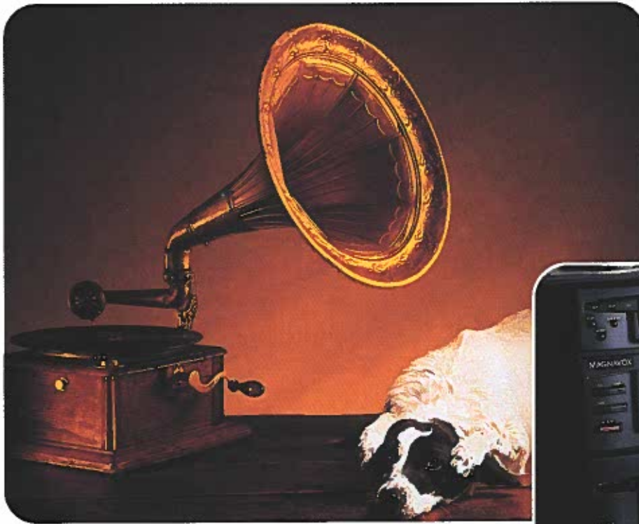
Fig. 2-5. Have you ever seen a phonograph like the one shown here? Manufactured around 1900, this model reproduced sound by means of a needle that followed a groove in a rotating disk, called a "record." Does the phonograph seem completely different from the CD player? Research how CDs are made and compare the two.
