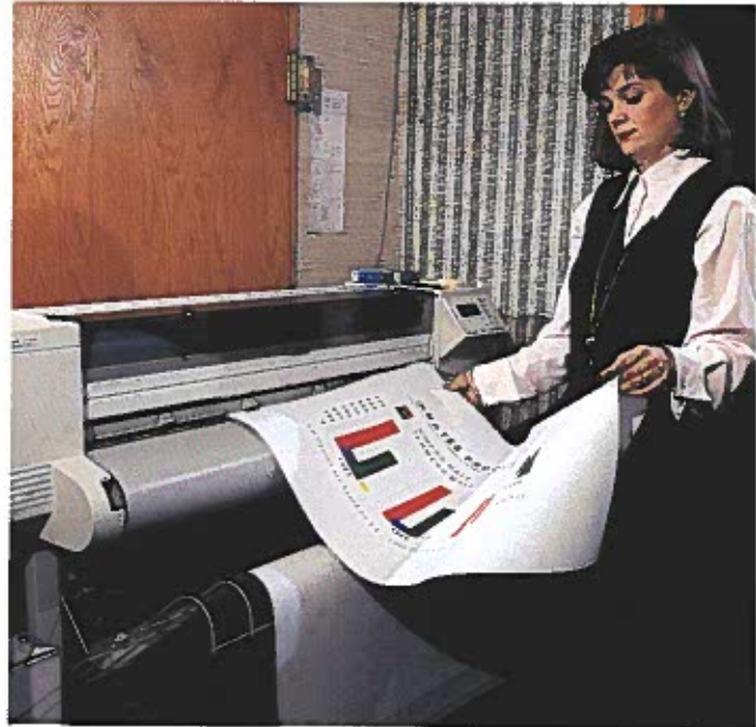
Fig. 5-6. This plotter is used to produce large drawings. What kinds of drawings might need to be this large?
