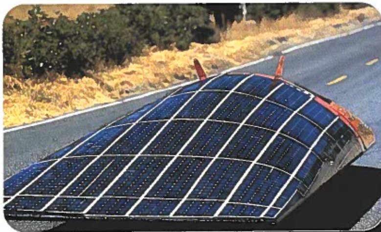
Fig. 7-5. The solar car (top) has photovoltaic cells in its roof. The sun provides the energy. The state of Iowa helps conserve energy by using flexible fuel vehicles (bottom) that run on blends of gasoline and up to 85 percent ethanol (an alcohol made from grains). Which service stations in your community sell ethanol blends?
