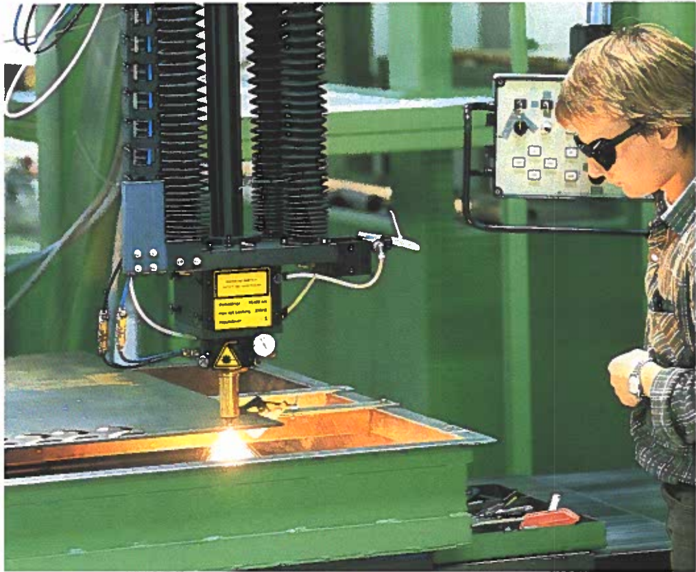
Fig. 7-8. A laser is an intensely focused beam of light. Here a laser is used to cut metal. Name some other uses for lasers.
