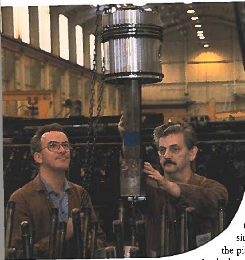
Fig. 8-11. Hydraulic pistons are used in locomotives. Why do you think they are so large?
