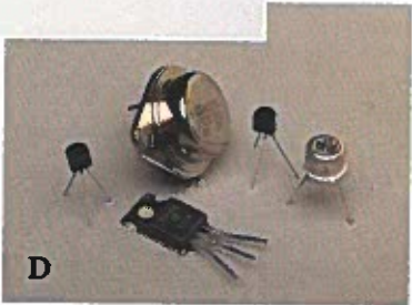
Fig. 8-9. Electronic components include (A) resistors, (B) capacitors, (C) diodes, and (D) transistors.
