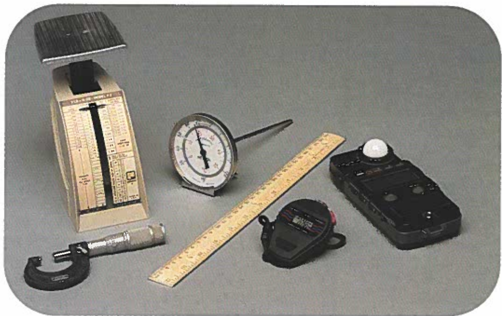
Fig. 9-1. These measuring instruments include (from left to right) a micrometer, scale, cooking thermometer, ruler, stopwatch, and photographic light meter.
