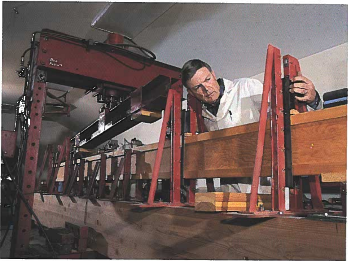
Fig. 9-9. This engineered-wood beam will be tested for compression strength. The metal beam will press down on top of the wooden one. Why do you think a beam would need to withstand compression?
