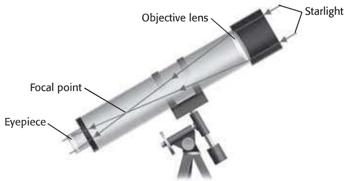
This simple refracting telescope has an objective lens that collects light and a lens in the eyepiece to magnify the image.
